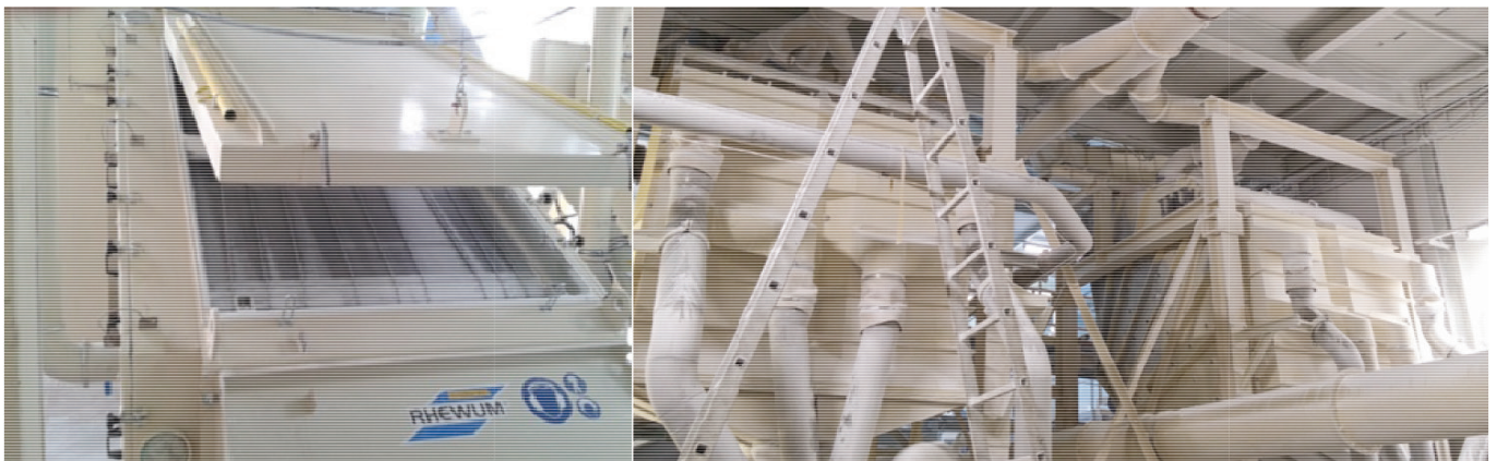
Figure 3 : RHEWUM sifter in the sugar industry (source: RHEWUM)
