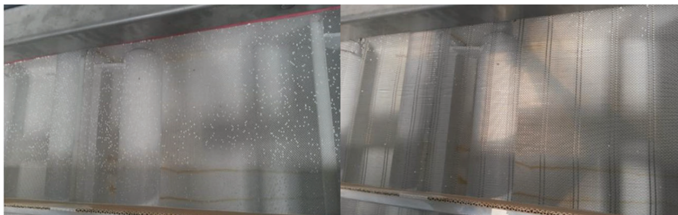
Figure 1 : Illustrates a clogged screen mesh with as quare opening in the fertiliser industry (on the left), which has been improved by the use of rectangular screen mesh openings (on the right) (source: RHEWUM)
